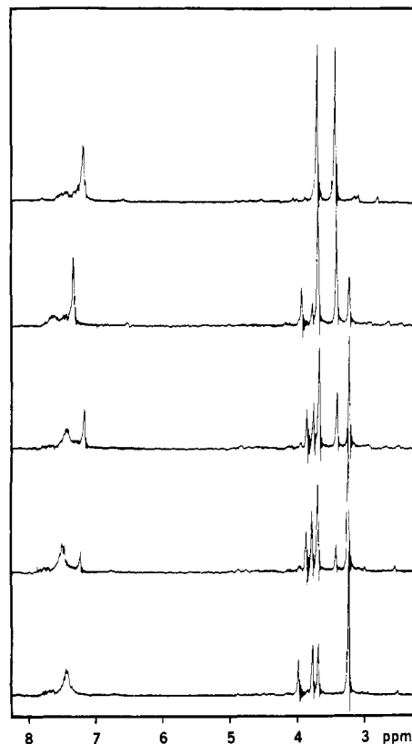
Figure 2. ^1\text{H} NMR spectra for the phosphorane 2b . The top spectrum has been recorded in \text{CDCl}_3 , and the doublet at \delta 3.6 represents the four equivalent \text{CH}_2 groups. The remaining spectra have been recorded in 0.005 M NaOD/ \text{D}_2\text{O} (HOD resonance at \delta 4) at approximately 30 s, 2 min, 5 min, and 15 min after phosphorane addition. The bottom spectrum represents the diester 4b and is characterized by a \text{CH}_2 doublet at \delta 3.7 ( \text{POCH}_2 ) and a \text{CH}_2 singlet at \delta 3.2 ( \text{CH}_2\text{OH} ).
